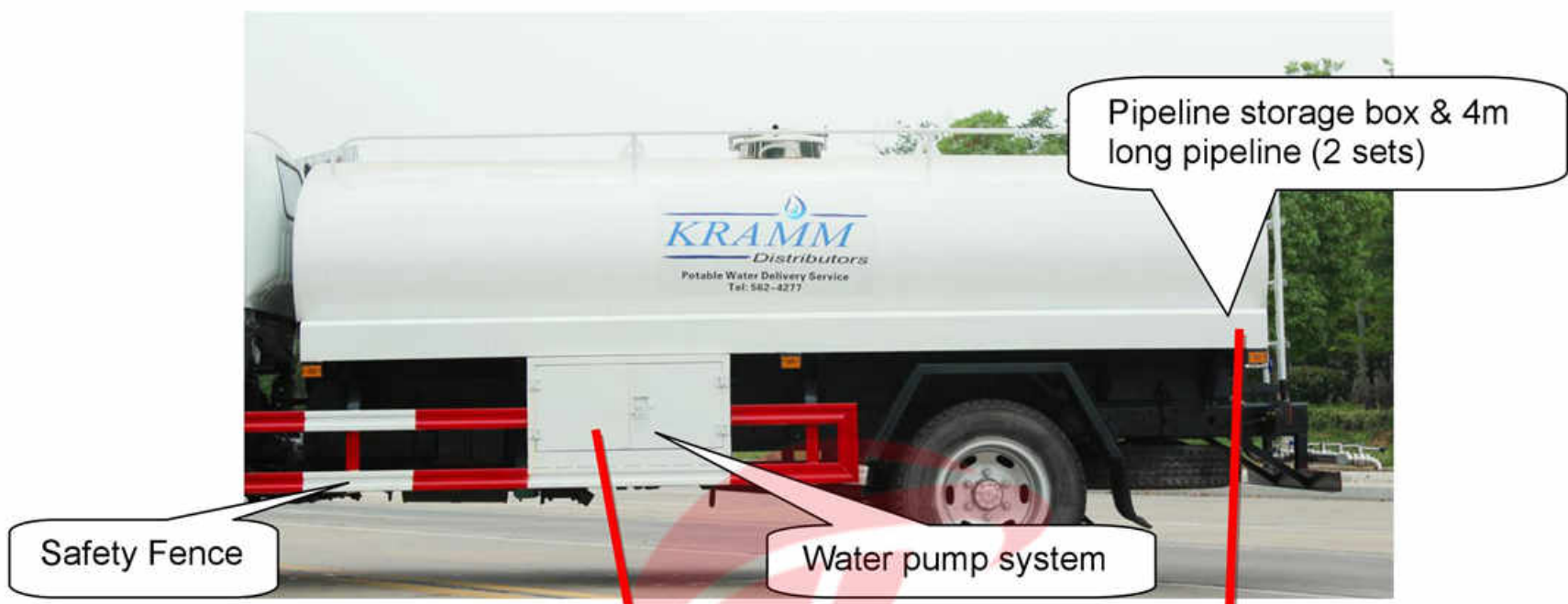
Left side of the Tank (Driver side): Water pump system, pipeline storage box and Safety fence
